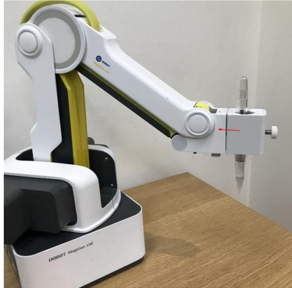
Figure 5.34 Install a writing and drawing kit
