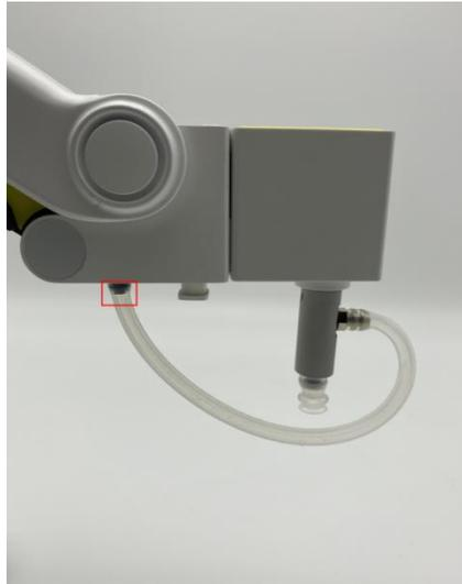
Figure 5.68 Install an air tube
