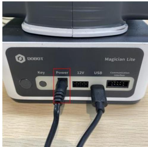
Figure 3.2 Connect Magician Lite to the electrical outlet
