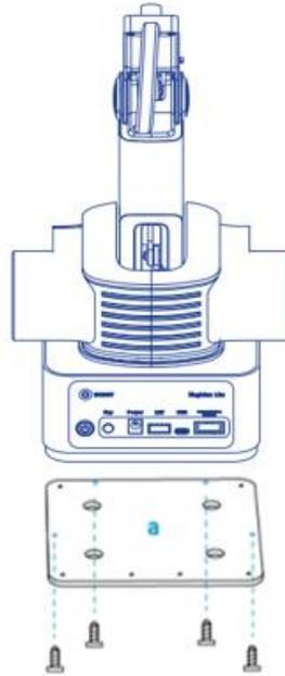
Figure 5.45 Fix plate a
