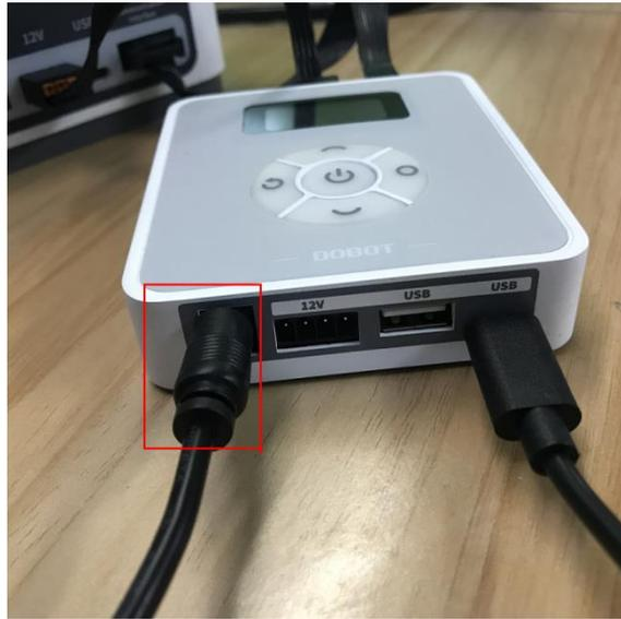
Figure 3.5 Connect power adapter
