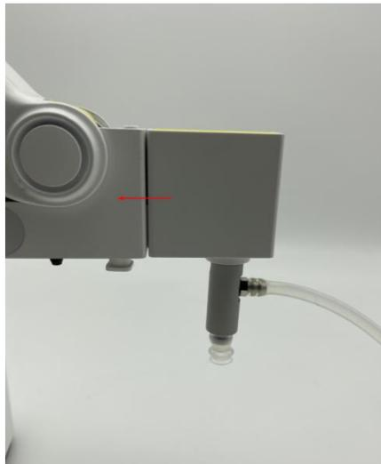
Figure 5.67 Install a suction cup kit
